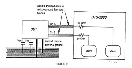
The DTS input termination levels are programmable from -3V to +3V. See figure 9. The common mode input operating range of the DTS is shown in figure 10. The input termination resistance is 50-ohms to the termination voltage.
