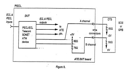
Figure 8 shows a PECL-to-ground reference level shifter. Chip resistors and capacitors minimize parasitic reactance. High quality  $50\Omega$  coax cable is required to transfer signals to the time measurement instrument.
