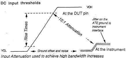
Input Attenuation used to achieve high bandwidth increases input errors due to DC voltage reference and instrument to ATE ground offsets.
