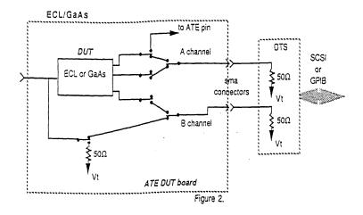
Current mode ECL and ECL-compatible GaAs are usually resistive terminated (anywhere from 50 to 100 ohms to -2 to +3 volts). The -3 volt devices are called PECL or Positive ECL. Some Telecom SDH clock recovery devices work with all three ECL terminations: -2, ground and +3 volts depending on how they are configured.
