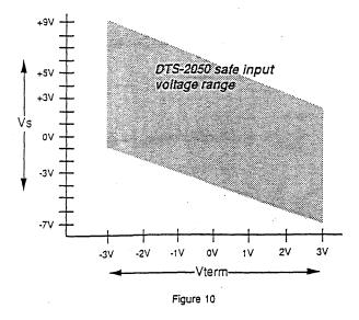
Figure 11 shows the power supply voltage relationships of the DTS to the DUT for GND termination and -2V termination. The safe input compliance of the DTS 2050 is -7V to +3V when the termination supply is set to +3.0 Volts. For PECL logic, use the level shifting scheme shown in figure 8.
