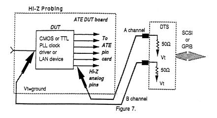
Active probing may be necessary for devices that cannot tolerate any type of current loading. High voltage swing linear functions with high internal series resistance usually require some form of active interface to buffer the DUT to ATE or external instrument. Refer to references 3 and 4 for details on high impedance active probe design considerations.
