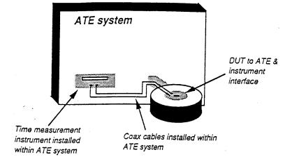
LSI and VLSI ATE systems normally have room within the confines of the system cabinets for external instruments. Most of these systems also have high quality  $50\Omega$  coax cables running between the instruments and test-head load-board interface hardware. Some systems have special coax pogo-pins to make contact to the DUT board. This level of integration is recommended for an accurate low jitter production and engineering environment.
